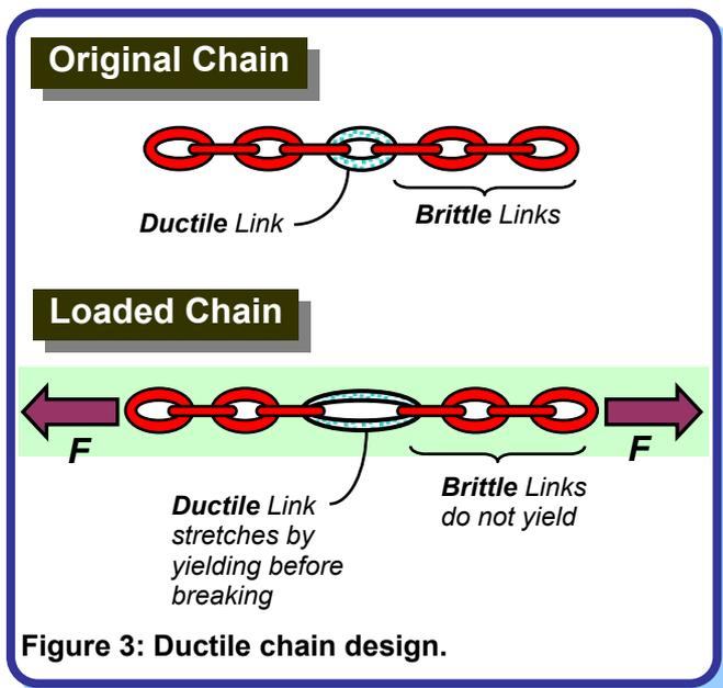
Figure 3: Ductile chain design.
