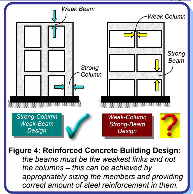
Figure 4: Reinforced Concrete Building Design: the beams must be the weakest links and not the columns – this can be achieved by appropriately sizing the members and providing correct amount of steel reinforcement in them.
