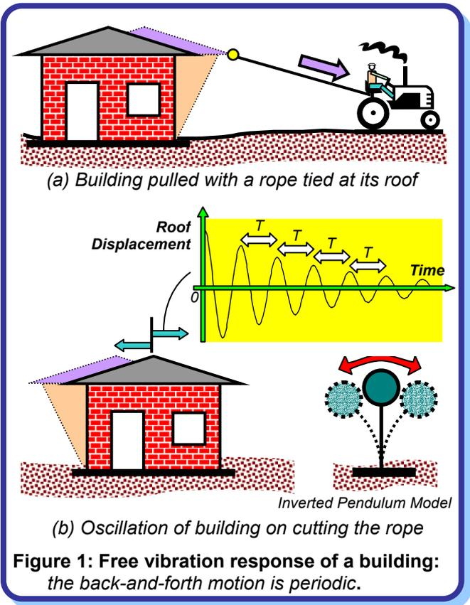
Fundamental natural period *T* is an inherent property of a building. Any alterations made to the building will change its *T*. Fundamental natural periods *T* of normal single storey to 20 storey buildings are usually in the range 0.05-2.00 sec. Some examples of natural periods of different structures are shown in Figure 2.
